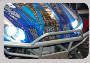
Rigid Industries HID kits are 100% plug and play using OEM connectors for quick and easy installation. We use the same aircraft digital ballast in every kit for low startup draw and almost no RFI emissions ensuring crystal clear stereo's and communication radios.
